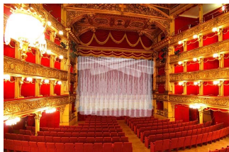
Test of a water mist curtain Spray-tecs for the protection of a theater curtain and the surrounding décor.
