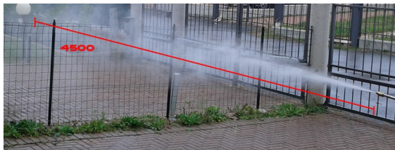
Test of a water mist nozzle for the protection of a tiny zone, positioned far from the nozzle.
